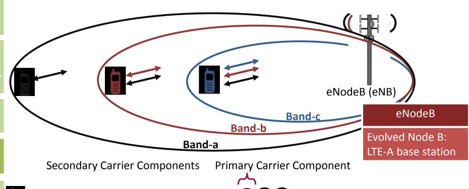
Up to 5 Carrier Components (CC) for downlink and uplink
