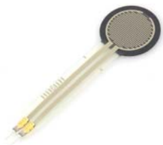
Fig. 2: Round Force Sensitive Resistor [31].
