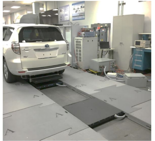
Fig. 2. The experimental of the passage of an EV through a two-coil track [27].
